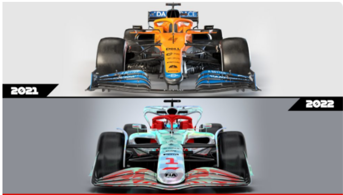
Figure 4: 2021 and 2022 Formula 1 Front Wings [F1T21]
